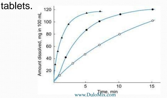
Rate of dissolution of phenacetin from ▲ powder, ● granules, and ○ tablet in diluted gastric juice.
